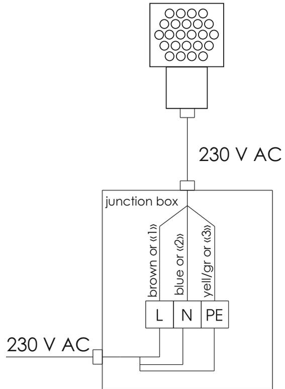
RAY color dynamic luminaire connections diagram
