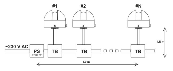
Line aggregate length (L0+L1+..+LN) < 500m.
